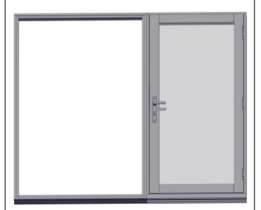
Fully support and carefully flip the unit over to install the interior mull.
