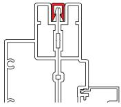
Cut the C-mull keys to the length on the exterior side of the unit. Install the mull with a mallets by tapping the mull key into the tracks. This will lock them together as shown above. You may need a block and hammer to drive the mull key in place. 10
