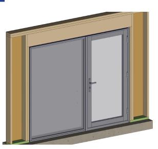
Install the mulled unit per standard installation guides. Swing door refer to IG-084. Sliding door refer to IG-085
