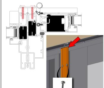
Place the interior mull (Die #: M25407) on to the face of the door. Drill a hole 11/64" hole through the wood and the aluminum leg. Drill a hole in each die line, 3" from each end and then 16" on center, as shown above. Then install fasteners #10, 1.25", (Part #: 0171859).
