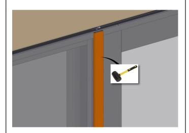
Take the interior mull cover (Die #: M25408) and snap it over the interior mull to cover fasteners.
