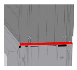
Cover the joint at the head and sill with sealant and tool flat as shown above.
