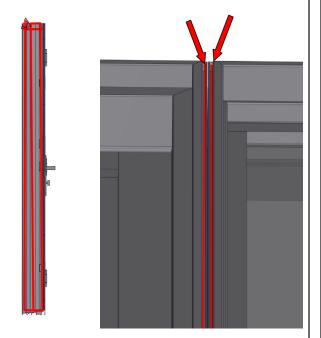
Apply silicone to the connecting sides of the unit. Run 3, 3/8" beads of silicone along the mulled side of the unit, also run a bead of silicone down each c-mull track that will be joined together.
