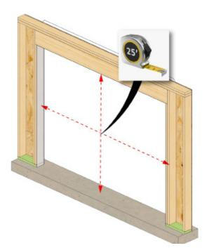
Measure and verify the rough opening is sized correctly. The rough opening should be 3/4" wider and 1/2" taller than the unit. Allow additional space for flashing thickness, installation clips, joining components, and their fasteners.
