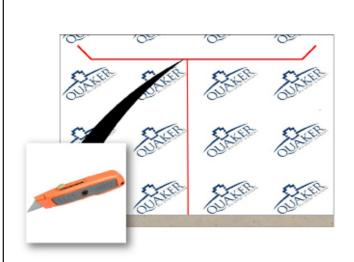
Apply the house wrap according to the manufacturer's instructions and cut T-pattern opening as shown above. Cut top flap angles at 45 degrees and 1" longer than the width of flashing tape being used.
