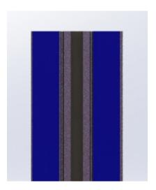
Cut the structural mull 3/8" less than window unit on units without the j-channel pocket. Cut the mull 2" less than window unit on units with the j-channel pocket. Clean structural mull with alcohol to remove any oil. Apply two strips of double-sided tape to both sides of mull.
