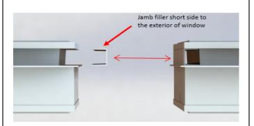
Install the j-channel filler into j-channel slot on the side to be mulled of the exterior of each window. Cut the filler short of head and sill j-channel slot so as not to obstructed the channel.
