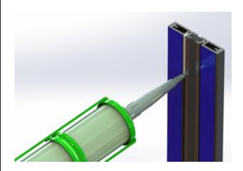
Apply a continuous bead of sealant to the ½" structural mull groove that will set over the cut down nail fin as shown above. Peel backing off the double-sided tape.
