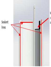
Make sure excess weld is clean for the jamb filler to set flush
