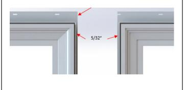
Using a utility knife score and remove all but 5/32" of the nailing fin from each unit where the mull will connect them. Make sure to cut the head and sill nail fins back flush with ripped nail fin.
