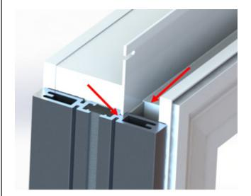
Apply the mullion to the side of the window aligning the groove in the mullion with the cut down nail fin. Make sure the mullion doesn't stick pass the j-channel pocket. Press firmly to engage the double-sided tape.
