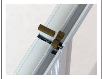
Insert foam plugs or backer rod into mull gaps at both ends of mullion.
