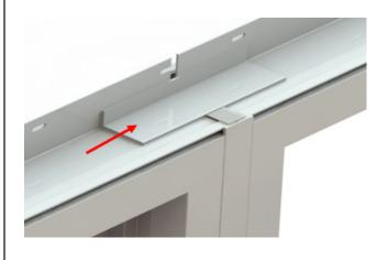
Apply 5"-7" piece of nail flange filler to interior back side of nail fin in a bed of sealant.
