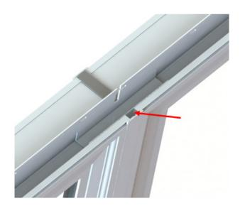
Apply sealant to the bottom edge of the jamb filler before installing it in the j-channel pocket at both ends of mullion, and add sealant to gap between filler and mull key.
