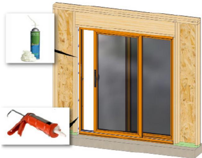
Fill interior 1/3 of cavity using low expanding foam or backer rod and apply sealant continuously around entire perimeter of opening.
