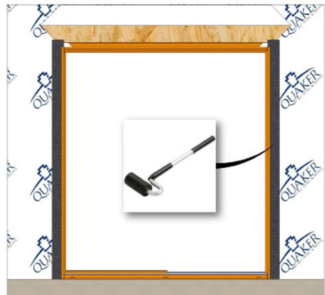
Apply flashing tape at the sides of the door as shown. Smooth using a J-roller. Extend tape a minimum of 2" past door frame, but not more than the thickness of the flashing tape.
