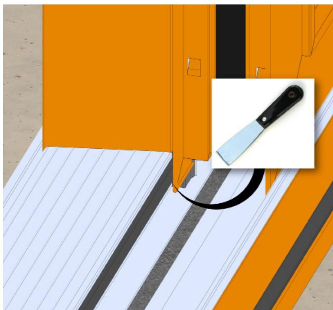
Slide active panel open all the way and use a putty knife to pull threshold cover weather strip up to help seal against
