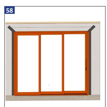
Unfold the house wrap top flap and tape the angled seams as shown.
