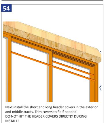
NOTE: ON ACTIVE PANEL MEASURE FROM PANEL TO FRAME AND SUBTRACT 1/16", CUT, THEN PLACE AGAINST FRAME.
