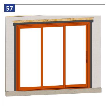
Apply a 3/8" sealant bead to the perimeter edge of door frame before installing the drip cap.
