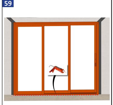
Apply a continuous bead of sealant at the exterior base of the sill. Be sure to not block the weeps on the bottom of the sill.
