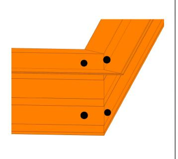
Start screws (Part #: FE FAST2) into the keys at each corner. Then tighten. Cover screws with silicone.
