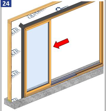
Slide the panel tight against the frame keeping the panel flush with the fixed panel extrusion in the sill.
