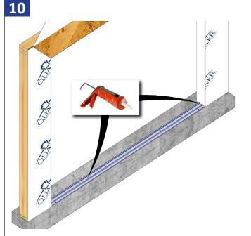
Apply sealant over fastener heads and at the ends of the sub-sill anchor plate where the plate meets the wall framing.
