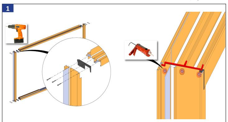
Apply the head and sill gaskets to each end of the head and sill. Assemble jambs to head and sill assembly with the 12 fasteners provided (MH8-18X11/2 LP) and seal around all screw heads, exposed screw threads, and outside corners.
