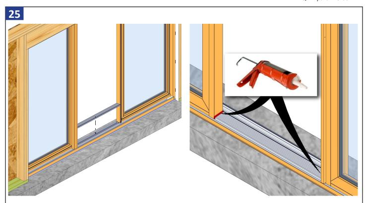
Install threshold on the exterior side of frame covering the bottom angle brackets. Seal around the two ends of the threshold against the frame.
