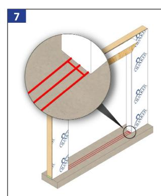
The sub-sill anchor plate will set 4 1/16" in from the exterior face of wall framing. Apply three 3/8" continuous beads of sealant across the entire width of the rough opening sill where the sub-sill anchor plate will set. Apply two 3/8" continuous beads of sealant the depth of the anchor plate, 1/2" from each side of opening as shown above.
