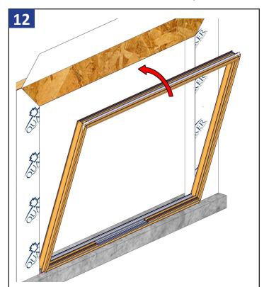
Center and set the door frame into the rough opening, making sure there are equal gaps on both sides of the door.
