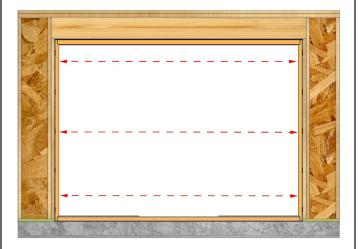
Check that the door frame is not bowed. Adjust shims as needed until measurements are within 1/8". Finish fastening the unit every hole or a minium of 12" on center.
