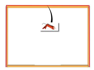
Apply a continuous 3/8" diameter bead of sealant along the backside of the nailing flange. Bead must run around both sides and across the head, in line with and completely covering the nail flange holes.
