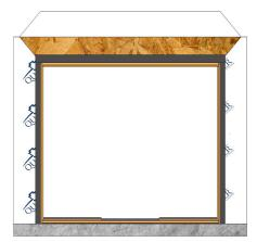
Apply a  $3/8^{\prime\prime}$  sealant bead to the top exterior edge of door frame before installing the drip cap.
