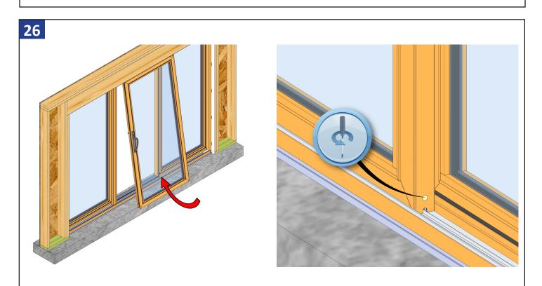
Angle the active panel with the top inserted into the head track, and then lift and set the bottom rollers on the roller track. Use a Phillips #3 screwdriver to adjust the rollers as needed to ensure the panel is level, square, and slides smoothly. Lift on the panel while adjusting, do not use a drill to adjust.
