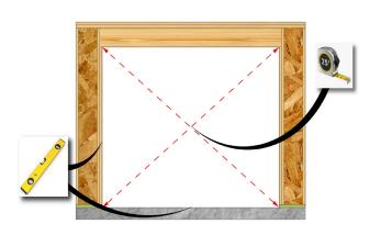
Check that the opening is square. The diagonal measurements need to be within 1/8" of each other. Verify the rough opening is plumb and level.
