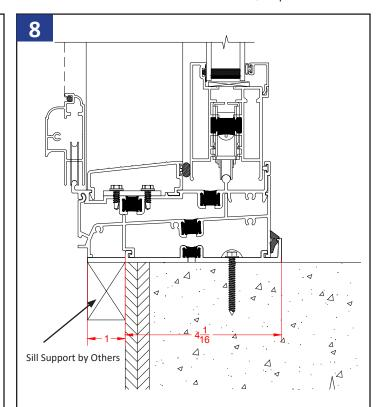
Install the sub-sill anchor plate 4 1/16" in from the exterior face of wall framing.
