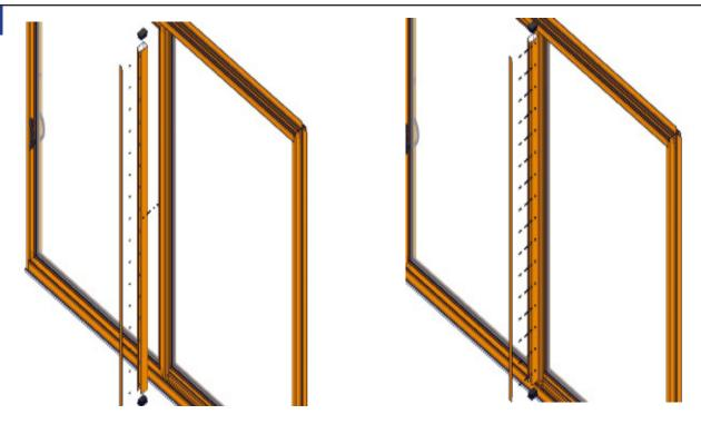
If reinforcement tube is to be applied, center the reinforcing tube on the active panel's meeting rail, and install using supplied (MH8-18x1/2 TK2) screws.
