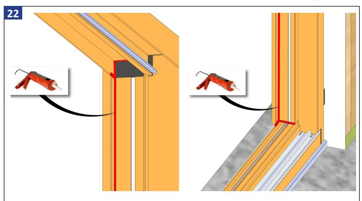
Seal the inside edge corners at the head, sill, and jamb where the fixed panel will set in the frame, as shown above.
