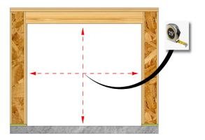
Measure and verify the rough opening is sized correctly. The rough opening should be 3/4" wider and 1/2" taller than the unit. Allow additional space for flashing thickness, installation clips, joining components, and their fasteners.
