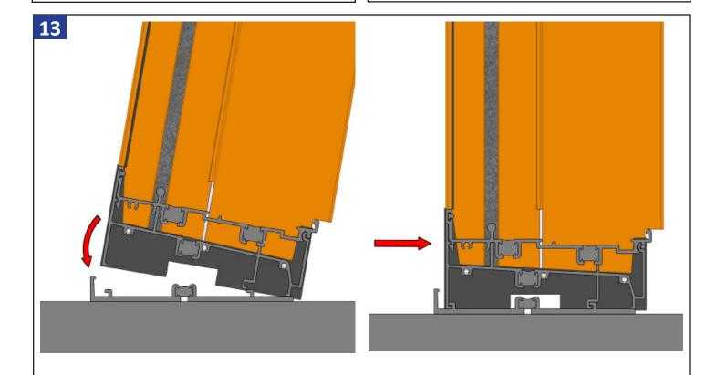
Angle the door frame with the top tilted out, and set the exterior sill frame inside the exterior leg of the sub-sill anchor plate as shown above. Tilt the door frame in against the wall framing, and push the sill out to lock the sill into the sub-sill anchor plate.
