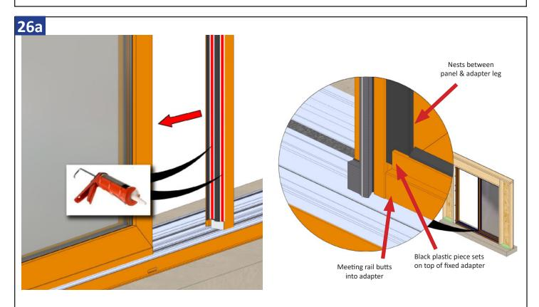
Apply a bead of sealant to inside edges of meeting rail before sliding the pre-assembled meeting rail against the fixed panel. Please see steps 26b and 26c for series specific guidelines.
