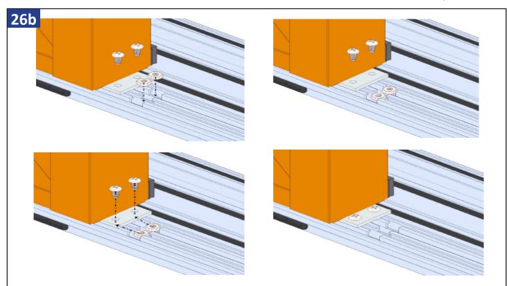
For ModernVu and M204 units, install the meeting rail using supplied (MH8-18X1/2 TK2) screws in the head, and (MP10/24X3/8 & 10-24 NUT) screws and nuts in the sill angle brackets. Repeat for other meeting rail.
