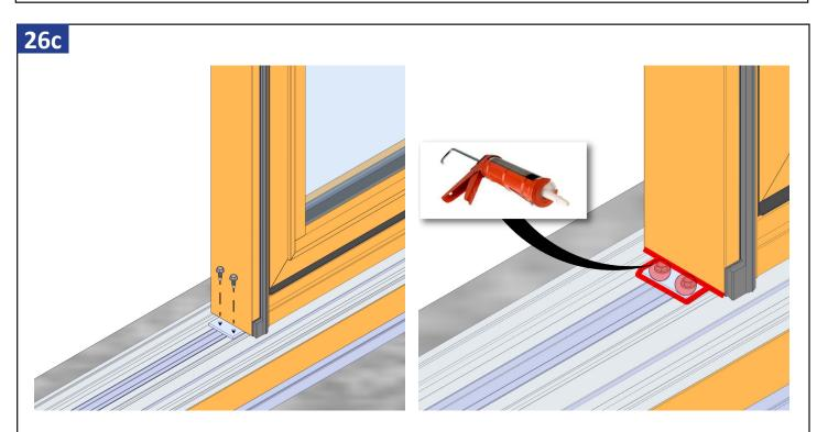
For all other M-Series units, install the pre-assembled meeting rail against the fixed panel and install using supplied (MH8-18X1/2 TK2) screws in the head and sill angle brackets. Apply sealant over the screw heads in the sill and along the perimeter of the angle bracket.
