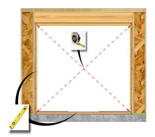
Check that the door is square. Adjust shims as needed until diagonal measurements are within 1/8". Level at the sill and plumb the frame.
