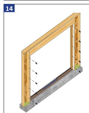
Shim at the sides of the door, and at the lock location as shown above. Never shim at the head.
