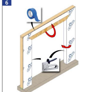
Fold the house wrap around the jambs to the interior and staple it to the interior framing. Fold the house wrap flap up and temporarily tape it in place.
