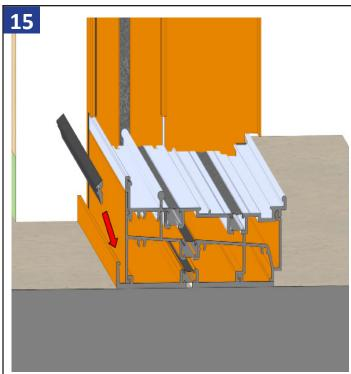
Install the wedge gasket in the sub-sill anchor plate against the interior leg of the door as shown above.
