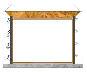
Apply flashing tape at the sides of the door as shown. Smooth using a J-roller. Extend tape a minimum of 2" past door frame, but not more than the thickness of the flashing tape.
