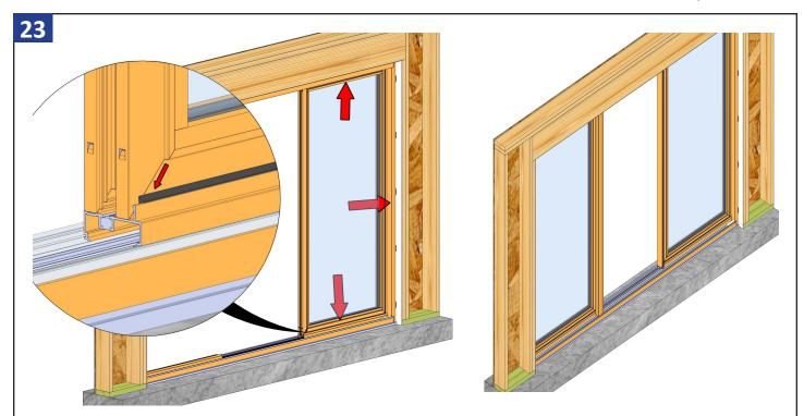
Install wedge gasket in the sill, head, and jamb around the interior of the frame and panel to secure the panel in place. Repeat steps 20, 21, 22, and the first step of 23 for the other stationary panel.
