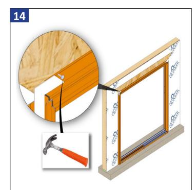
Temporarily tack the door into place using 2" galvanized roofing nails through the pre-punched holes on one top corner of the nailing flange.
