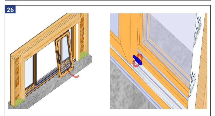
Angle the active panel with the top inserted into the head track, and then lift and set the bottom rollers on the roller track. Use a Phillips #3 screwdriver to adjust the rollers as needed to ensure the panel is level, square, and slides smoothly. Lift on the panel while adjusting, do not use a drill to adjust.
