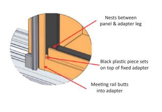
Apply a bead of sealant to inside edges of meeting rail before sliding the pre-assembled meeting rail against the fixed panel. Please see steps 24b and 24c for series specific guidelines.
