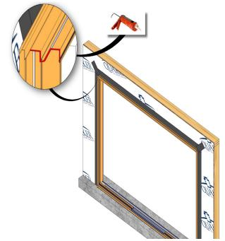
Seal the inside edge corners at the head and sill where the fixed panel will set in the frame.
