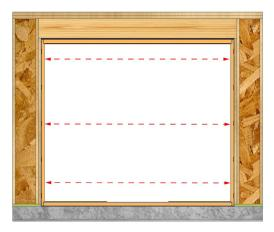
Check that the door frame is not bowed. Adjust shims as needed until measurements are within 1/8". Finish fastening the unit every hole or a minium of 12" on center.
