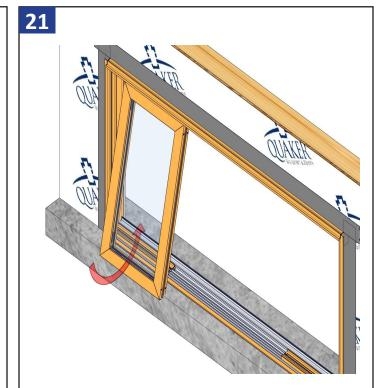
Angle the fixed panel with the top inserted into the head track, and then lift and set the bottom of the panel on the fixed panel extrusion in the sill.
