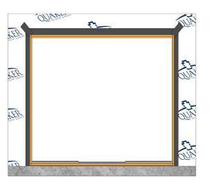
Unfold the house wrap top flap and tape the angled seams as shown.
