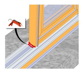
For all other M-Series units, install the pre-assembled meeting rail against the fixed panel and install using supplied (MH8-18X1/2 TK2) screws in the head and sill angle brackets.
