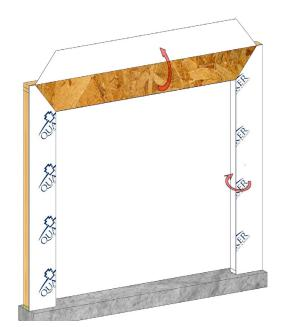
Fold the house wrap to the interior and staple it to the interior framing. Fold the house wrap flap up and temporarily tape it in place.
