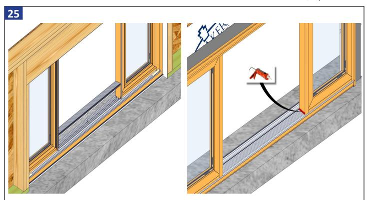
Install threshold on the exterior side of frame covering the bottom L-angle bracket. Seal around the two ends of the threshold against the frame.
