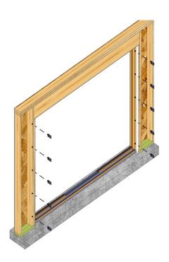
Shim at the sides of the door, and at the lock location as shown above. Never shim at the head.
