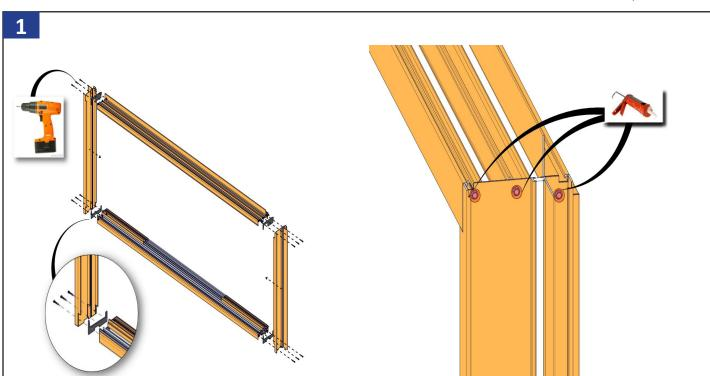
Assemble jambs to head and sill assembly with the 12 fasteners provided (MH8-18X11/2 LP). Make sure to use the two head and sill gaskets provided, and seal around screw heads and outside corners.
