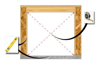
Check that the opening is square. The diagonal measurements need to be within 1/8" of each other. Verify the rough opening is plumb and level. The sill plate beneath the unit must be level for proper unit operation.
