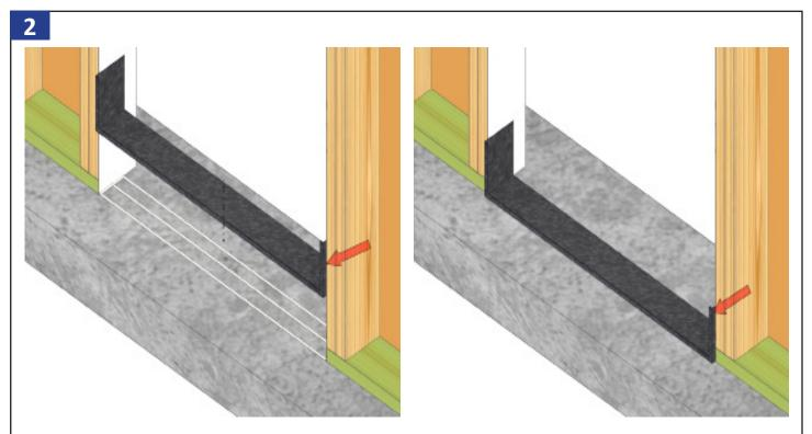
Install a sill pan flashing (by others). If installing the door flush with the interior to allow for a 180 degree door swing make sure to set the sill pan flush with interior wall finish.
