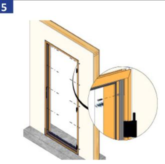
Drill a countersink hole through the jambs in the exterior track per anchorage calculations. *Quaker Window Products does not supply or claim liability for anchorage/fastener calculations. It is the installer/client's responsibility for structural adequacy of the anchorage and fasteners.* Typically, 3" from the corners and 16" on center, and at every hinge and lock location.
