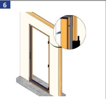
Install and fasten the door unit in place using fasteners by others per anchorage calculations. *Quaker Window Products does not supply or claim liability for anchorage/ fastener calculations. It is the installer/client's responsibility for structural adequacy of the anchorage and fasteners.* Typically, 3" from the corners and 16" on center, and at every hinge and lock location.
