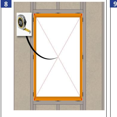
Check that the window is square. Adjust shims as needed until diagonal measurements are within 1/8".
