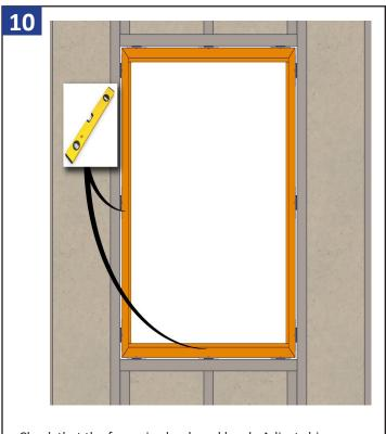
Check that the frame is plumb and level. Adjust shims as needed.
