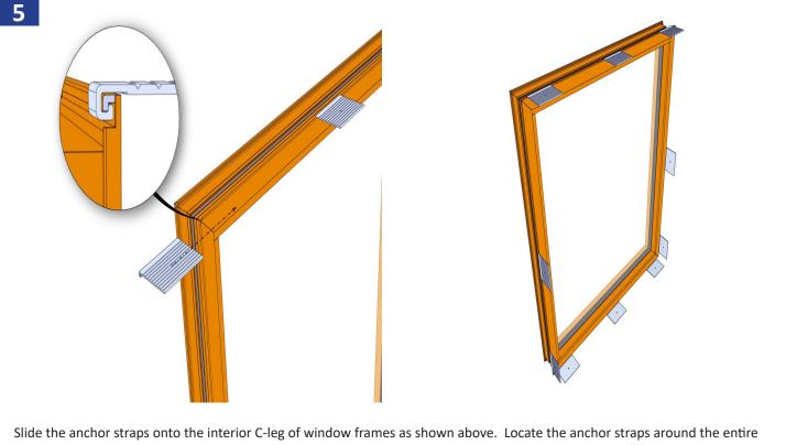
Slide the anchor straps onto the interior C-leg of window frames as shown above. Locate the anchor straps around the entire window perimeter positioned as noted on the shop drawings and or anchorage calculations. Typically 3" from the corners and 12" on center.
