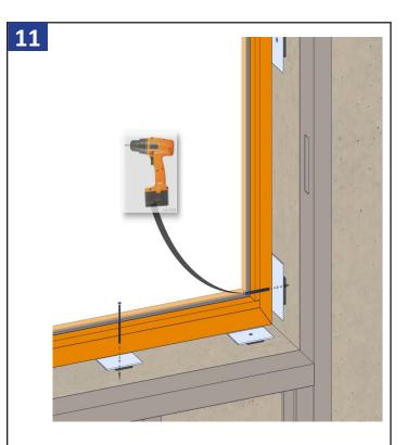
Finish fastening the unit using a minimum of one screw per anchor strap.
