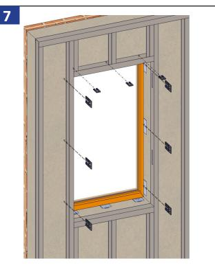
Shim at the sides of the window, and the check rail locations. Make sure to shim the window and the backside of the anchor straps.
