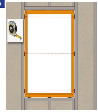
Check that the window is not bowed. Adjust shims as needed until measurements are within 1/8".
