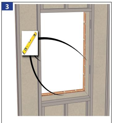
Verify the rough opening is plumb and level. The sill plate beneath the unit must be level for proper unit operation.
