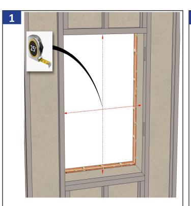
Measure and verify the opening is sized correctly. The rough opening should be a minimum 1/2'' (but not to exceed 1'') wider and taller than the unit. Allow additional space for flashing thickness, installation clips, joining components, and their fasteners.
