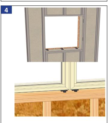
Place shims on the bottom of the opening under each side jamb location insert 1/4" from each side. If installing a mulled unit make sure to shim at all mull locations as shown above.
