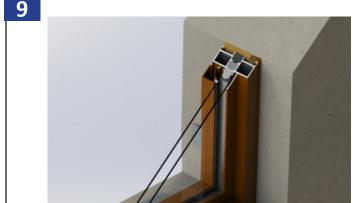
Operate window unit to ensure proper operation. Sash will not operate correctly if window is out of square, overshimmed or over-insulated. Allow foam to fully cure before installing interior trim. Install interior finish trim.
