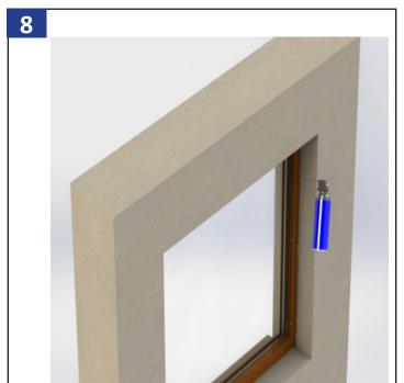
Insulate between the window frame and the rough opening using minimally expanding window and door spray foam or fiberglass insulation that is compliant with AAMA 812-04. Read and follow the manufacturers' recommendations for application and use.
