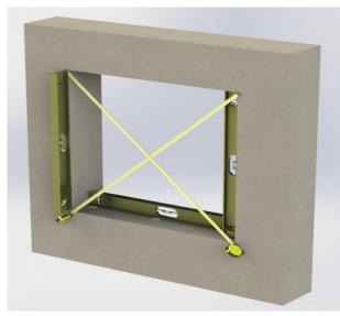
Measure and verify the size of the rough opening. The rough opening should be a minimum %" (but not to exceed 1") wider and taller than the unit. The masonry opening should be sized %" wider and 9/16" higher than the units exterior frame. Verify the rough opening is flat, plumb, level, and square. Take diagonal measurements to check for square.
