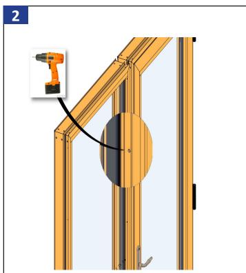
Predrill holes in jamb for #8 screws to attach mull #57588 3" from top and bottom and 16" on center thereafter.
