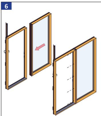
Install Side-lite and vertical mull into opening. Fasten door frame to mull using #8-1 3/4" screws.
