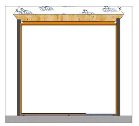
Apply flashing tape at the sides of the door as shown. Smooth using a J-roller. Extend tape a minimum of 2" pass window frame.
