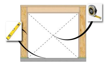
Measure and verify the opening is sized correctly. The rough opening should be a minimum 1/2" (but not to exceed 1") wider and taller than the unit. Allow additional space for flashing thickness, installation clips, joining components, and their fasteners.
