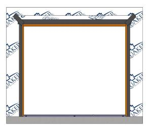
Unfold the house wrap top flap and tape the angled seams as shown.
