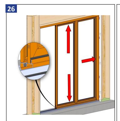
Install wedge gaskets in the sill, head, and jamb around the interior of the frame and panel to secure the panel in place.
