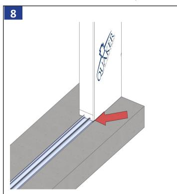
You'll need to cut the sill started to the rough opening. Install the sub-sill anchor plate keeping the exterior edge of sub-sill anchor plate in line with exterior of wall framing.
