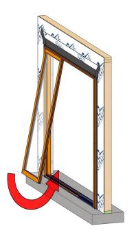
Angle the fixed panel with the top inserted into the head track, and then lift and set the bottom of the panel on the fixed panel extrusion in the sill.
