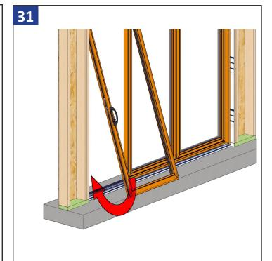
Angle the active panel with the top inseted into the head track, and then lift and set the bottom rollers on the roller track.
