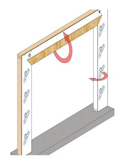
Fold the house wrap to the interior and staple it to the interior framing. Fold the house wrap flap up and temporarily tape it in place.
