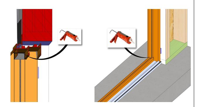
Seal the inside edge corners at the head and sill where the fixed panel will set in the frame.
