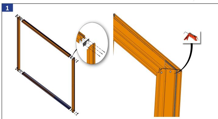
Assemble jambs to head and sill assembly with the 12 fasteners provided (MH8-18X11/2 LP). Make sure to use the two head and sill gaskets provided, and seal around all screw heads and outside corners.
