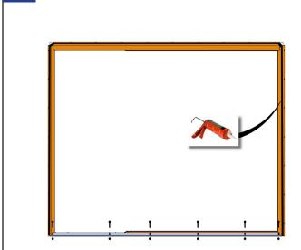
Apply a continuous 3/8" diameter bead of sealant along the backside of the nailing flange. Bead must run around both sides and across the head, in line with and completely covering the nail flange holes.
