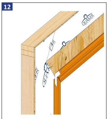
Temporarily tack the door into place using 2" galvanized roofing nails through the pre-punched hole on one top corner of nailing flange.
