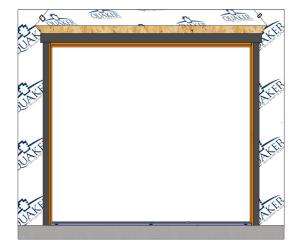
Apply a 3/8" sealant bead to the top exterior edge of door frame before installing the drip cap.
