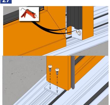
Apply a bead of sealant to inside edges of meeting rail before sliding the pre-assembled meeting rail against the fixed panel and install using supplied (MH8-18X1/2 TK2) screws in the head and sill angle brackets.
