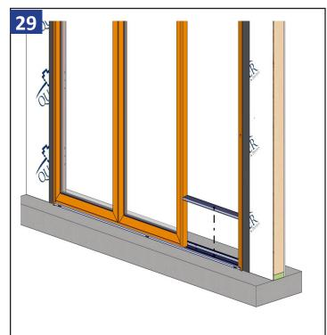
Install threshold on the exterior side of frame covering the bottom angle brackets.
