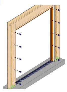
Shim at the sides of the door, and at the lock location as shown above. Never shim at the head.
