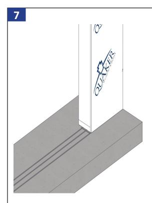
Apply three 3/8" continuous beads of silicone across the entire width of the rough opening sill, and a 3/8" continuous bead of silicone  $\frac{1}{2}$ " from each side of the rough opening as shown above.
