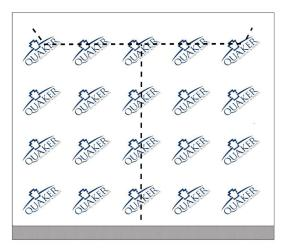
Apply the house wrap according to the manufacturer's instructions and cut T-pattern opening as shown above. Cut top flap angles at 45 degrees and 1" longer than the width of flashing tape being used.
