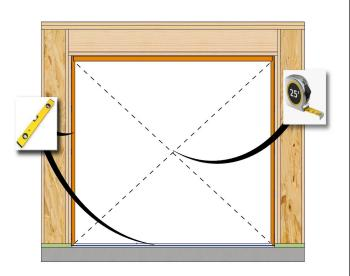
Check that the door is square. Adjust shims as needed until diagonal measurements are within 1/8". Level at the sill and plumb the frame.
