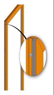
Second fixed panel will come with bridging astragal preinstalled with screws drilled through into the the panel thermofill
