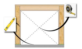
Check that the opening is square. The diagonal measurements need to be within 1/8" of each other. Verify the rough opening is plumb and level. The sill plate beneath the unit must be level for proper unit operation.
