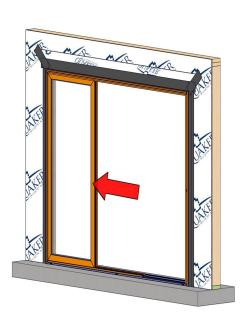
Slide the panel tight against the frame keeping the panel flush with the fixed panel extrusion in the sill.
