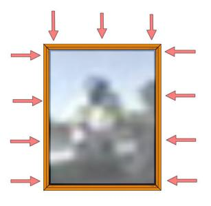
With the glass in the frame, install the remaining setting blocks around the glass perimeter. Place a block no more than 6 inches from each corner, and along the perimeter of the glass every 18 inches.
