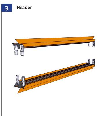
Repeat steps 1 and 2 for the header frame member. Both the header and sill members should have one gasket, 2 corner keys, and 2 key screws on each mitered end.
