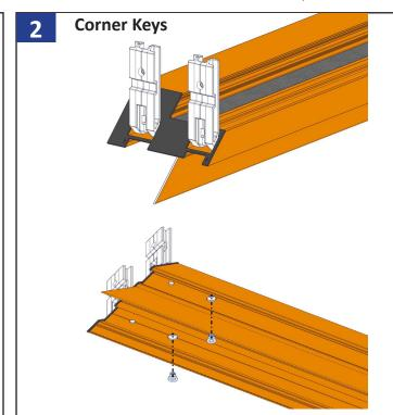
Insert and screw the corner keys into the ends of the sill frame with the provided corner key screws as shown. Each mitered end gets two keys, each key gets one screw through the frame piece.
