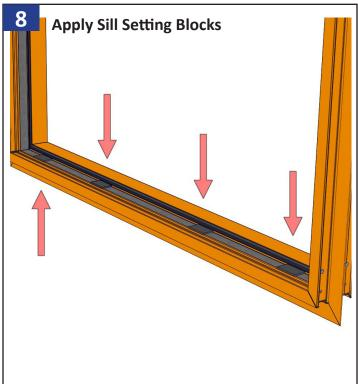
Insert provided setting blocks on the sill. Place 1 block in each corner no more than 6" from the jamb. Continue to place blocks along the sill spacing them no more than 18" apart.
