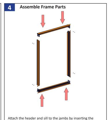
corner keys into the open ends of the jambs and screwing
