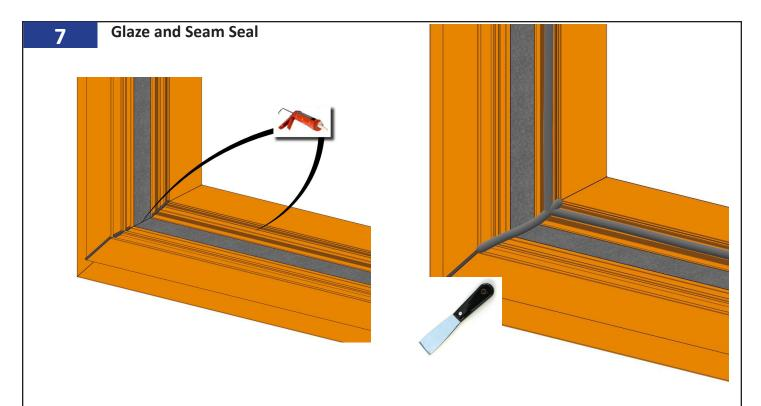
Apply a continuous 1/4" bead of sealant along the glazing legs filling the T-track. Then apply a bead of sealant along the inside corners of the frame from the glazing leg out to seal the seam. Tool the sealant in the corners.
