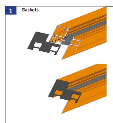
Starting with the sill frame, apply a gasket to each mitered end by placing the adhesive side of the gasket to the mitered end. Ensure the gasket slightly overlaps the perimeter.
