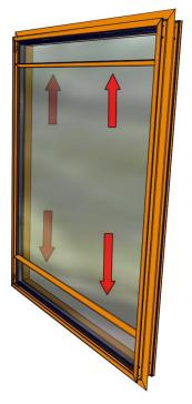
Install the horizontal glazing stops first at the head and sill, then install the vertical stops at the jambs to lock the glass into frame.
