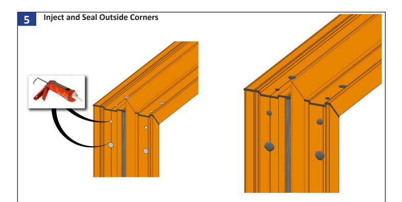
Using a caulk gun and sealant, inject sealant through the injection hole until the sealant can be seen through the other injection hole along that corner key. Also cover the screw heads for the corner key screws. Repeat for each corner key in entire assembly.
