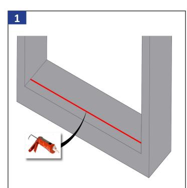
Apply a continuous bead of sealant that the U-Channel will sit on. Outside edge of U-Channel will be 1-9/16" from edge of opening. If sill is unlevel, shim if necessary.
