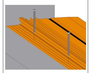
Set sill flashing on continuous bead of sealant. Screw sill flashing to anchor leg using fasteners per shop drawings or anchorage calculations. Screws are generally placed 3" off each end and every 12" in between.
