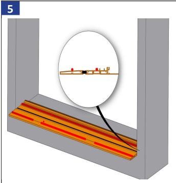
Apply a continuous bead of sealant into the track where the unit's interior edge will sit. Apply a broken bead of sealant for the exterior leg of the unit.
