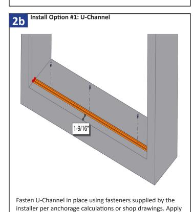
silicone between the U-Channel and wall at both ends. U-Channel exterior edge is 1-9/16" from the opening.
