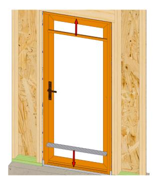
Install the jamb covers, then the head cover and threshold.
