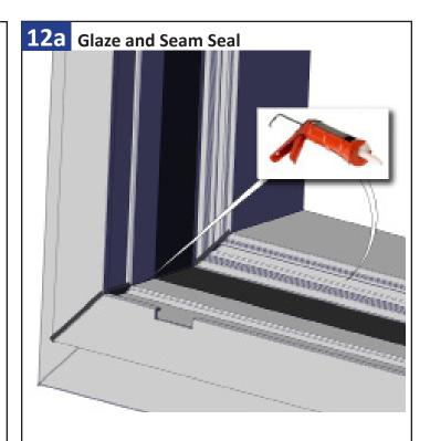
Apply a continuous 1/4" bead of sealant along the glazing legs filling the T-track. Then apply a bead of sealant along the inside corners of the frame from the glazing leg out to seal the seam. Tool the sealant in the corners.
