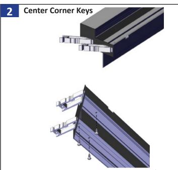
Insert and screw the center corner keys into the end of the sill frame with the provided corner key screws as shown.
