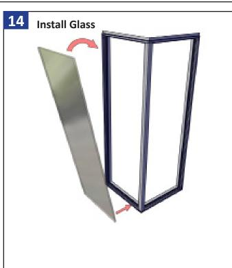
Install the insulating glass unit into the window frame from the exterior, bottom first and tilting the glass into the frame.
