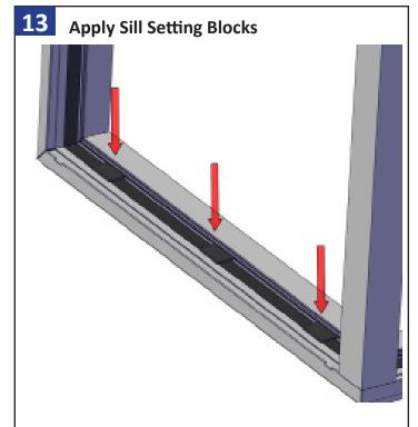
Insert provided setting blocks on the sill. Place 1 block in each corner no more than 2" from the jamb or TDL post. Continue to place blocks along the sill spacing them no more than 18" apart.
