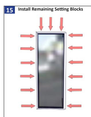
With the glass in the frame, install the remaining setting blocks around the glass perimeter. Place a block no more than 6 inches from each corner, and along the perimeter of the glass every 18 inches.
