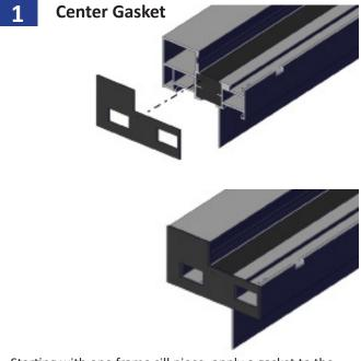
Starting with one frame sill piece, apply a gasket to the angled end by placing the adhesive side of the gasket to the frame. Ensure the gasket slightly overlaps the perimeter.
