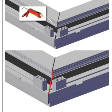
Apply sealant over the gasket as shown above for both the sill and head assemblies.
