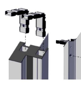
Insert and screw the corner keys into the ends of the jambs with the provided corner key screws as shown. Each jamb end gets 2 keys, each key gets one screw through the jamb.
