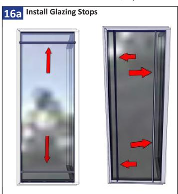
Install the horizontal glazing stops first at the head and sill,
