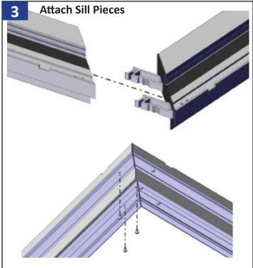
Attach the sill pieces together by sliding the center corner keys into the other sill piece and screwing in place.
