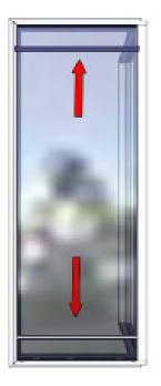
Install the horizontal glazing stops first at the head and sill. Then install the the 1 vertical stop.
