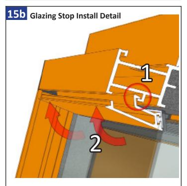
Install the stop by rolling the stop into place. A mallet may be required to persuade the stops to lock into place.
