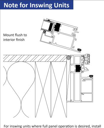
For inswing units where full panel operation is desired, instal the unit flush with interior finish surface of wall.
