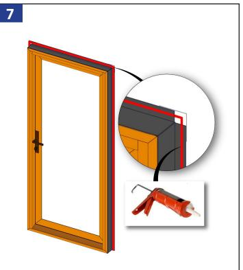
Apply a continuous 3/8" bead of sealant around the perimeter of the interior side of the positioning fin as shown.
