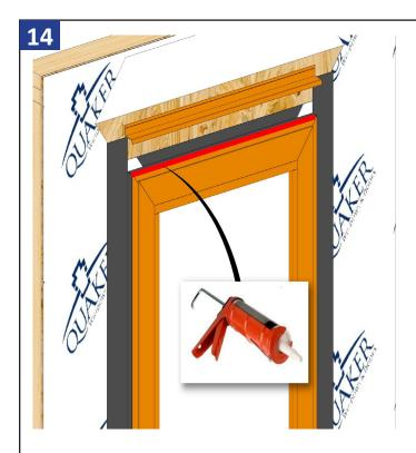
Apply a 3/8" bead of sealant to the top exterior edge of door frame before installing the drip cap as shown.
