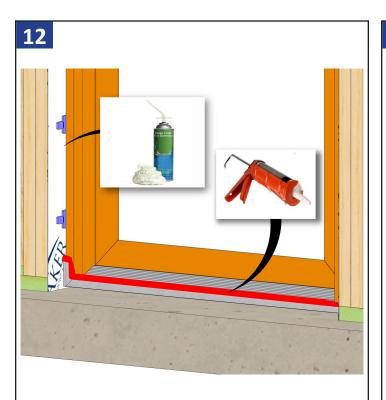
Apply a bead of sealant to fill the gap between the sill pan flashing system and the door unit. Make sure to seal all the way up both ends of the corner mold against the door. Insulate around the entire perimeter of the door.
