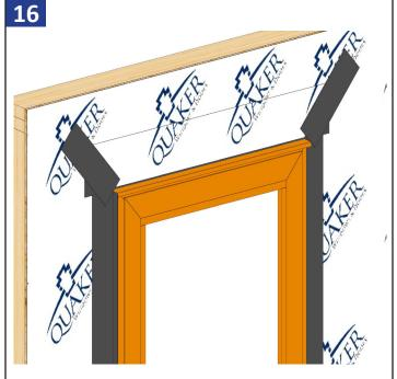
Flip down upper flap of the weather resistant barrier so it lays flat across head flashing and tape the angle cuts as shown above.
