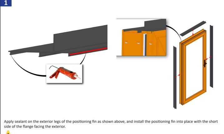
For best recommended results, apply and seal all positioning fins 24 hours prior to door installation.
