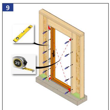
Square, level, and plumb unit in the rough opening by applying shims as needed. Shim behind all hinges and lock points, do not over shim, do not shim at the head.
