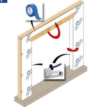
Fold the house wrap around the jambs to the interior and staple it to the interior framing. Fold the house wrap flap up and temporarily tape it in place.
