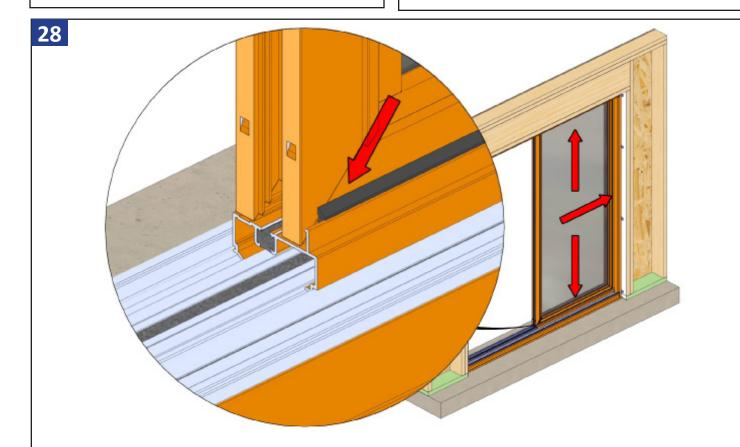
Install wedge gaskets in the sill, head, and jamb around the interior of the frame and panel to secure the panel in place.
