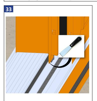
Slide active panel open all the way and use a putty knife to pull threshold cover weather strip up to help seal against the active panel.
