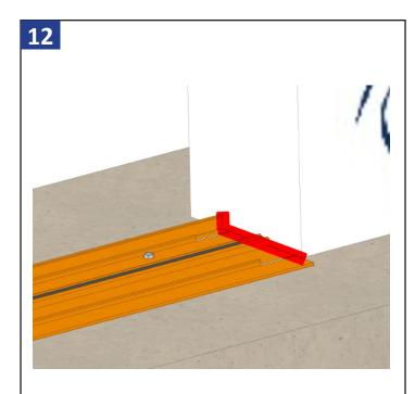
Be sure to run a bead of silicone across the plate and up the interior leg as shown above.
