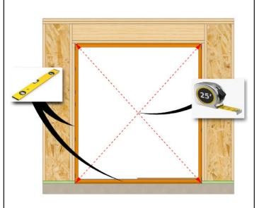
Check that the door is square. Adjust shims as needed until diagonal measurements are within 1/8". Level at the sill and plumb the frame.
