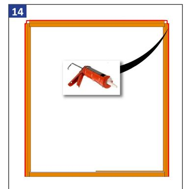
Apply a continuous 3/8" diameter bead of sealant along the backside of the nailing flange. Bead must run around both sides and across the head, in line with and completely covering the nail flange holes.
