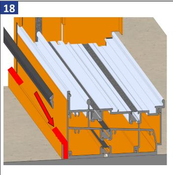
Run a 1" long bead of silicone completely filling the wedge gasket track at each end. Then install wedge gasket.
