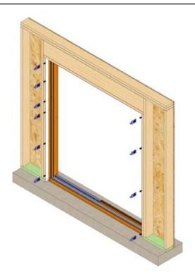
Shim at the sides of the door, and at the lock location as shown above. Never shim at the head.
