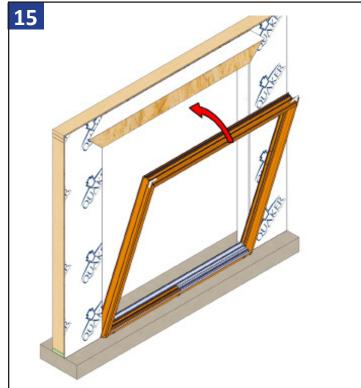
Center and set the door frame into the rough opening, making sure there are equal gaps on both sides of the door.
