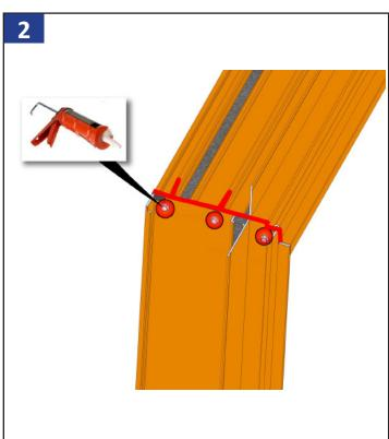
For KD and pre-assembled frames, seal around all screw heads, exposed screw threads, and outside corners.
