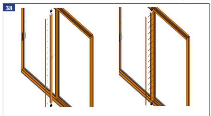
If reinforcement tube is to be applied, center the reinforcing tube on the active panel's meeting rail, and install using supplied (MH8-18x1/2 TK2) screws.
