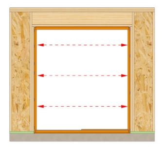
Check that the door frame is not bowed. Adjust shims as needed until measurements are within 1/8". Finish fastening the unit every hole or a minium of 12" on center.
