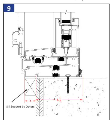
Install the sub-sill anchor plate 4 1/16" in from the exterior face of wall framing.
