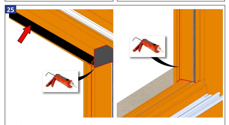
Place foam along head by removing the backing and stick along the leg as shown above. Seal the inside edge corners at the head, sill, and jamb where the fixed panel will set in the frame, as shown above.
