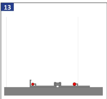
Run a continuous bead of sealant along each leg the entire width.
