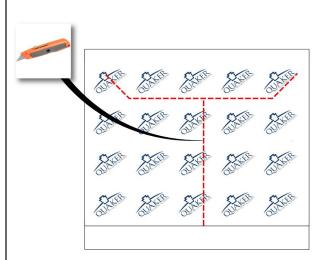
Apply the house wrap according to the manufacturer's instructions and cut T-pattern opening as shown. Cut top flap angles at 45 degrees and 1" longer than the width of flashing tape being used.
