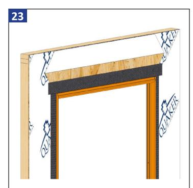
Apply a 3/8" sealant bead to the top exterior edge of door frame before installing the drip cap.
