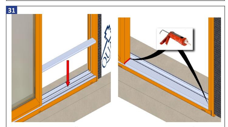
Install threshold on the exterior side of frame covering the bottom angle brackets. Seal around the two ends of the threshold against the frame as shown above.
