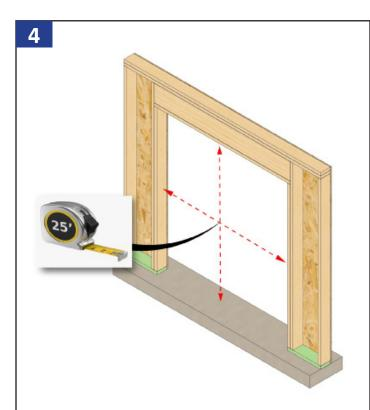
Measure and verify the rough opening is sized correctly. The rough opening should be 3/4" wider and 1/2" taller than the unit. Allow additional space for flashing thickness, installation clips, joining components, and their fasteners.
