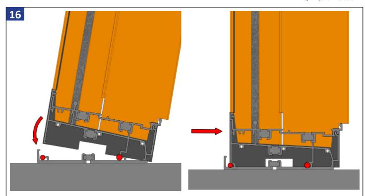
Angle the door frame with the top tilted out, and set the exterior sill frame inside the exterior leg of the sub-sill anchor plate as shown above. Tilt the door frame in against the wall framing, and push the sill out to lock the sill into the sub-sill anchor plate.
