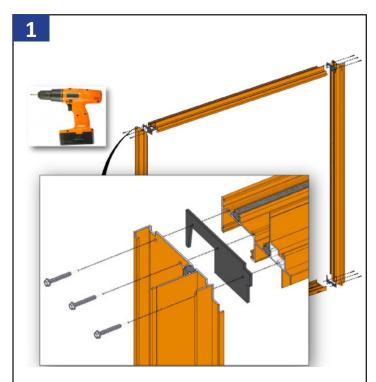
Apply the head and sill gaskets to each end of the head and sill. Assemble jambs to head and sill assembly with the 12 fasteners provided (MH8-18X11/2 LP) Install the jamb with the door keeper holes to the side of the sill that does not have the fixed panel adapter.
