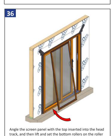
track. Adjust rollers as needed to insure the panel is level,
