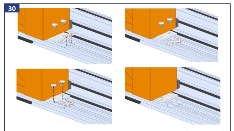
For M204 units, install the meeting rail using supplied (MH8-18X1/2 TK2) screws in the head, and (MP10/24X3/8 & 10-24 NUT) screws and nuts in the sill angle brackets.
