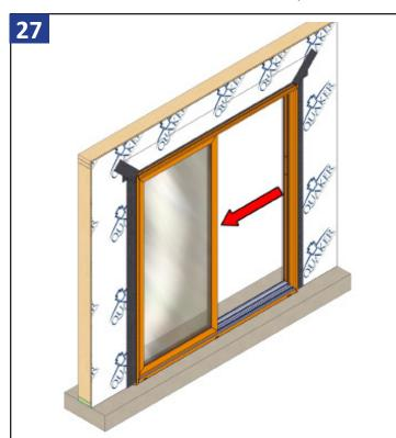
Slide the panel tight against the frame keeping the panel flush with the fixed panel extrusion in the sill.
