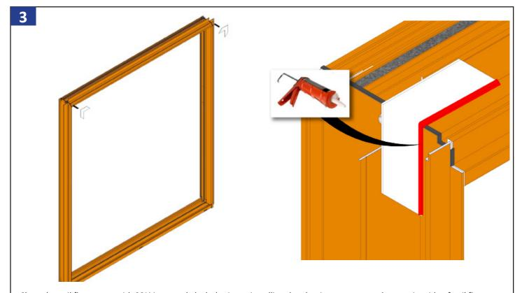
Clean the nail fin corners with 99% isopropyl alcohol prior to installing the aluminum corner to the exterior side of nail fin corner gaps. Apply sealant along the edge where the gasket meets the door frame as shown.
