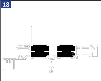
First drill a hole (11/32") through the frame, as shown above. Then take a 3/8" drill bit and drill through the first web making a clearance hole for the fasteners head clear. Install fasteners (Part #: MF#10-12X21/2).
