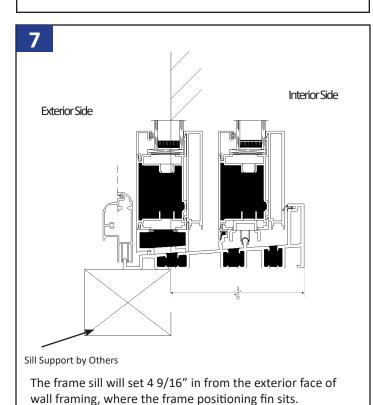
The unit must be supported the full width and
