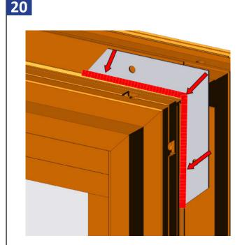
Remove backing off of the nail fin corner and attach the nail fin corner to the nail fins. Then silicone along the frame as shown above.
