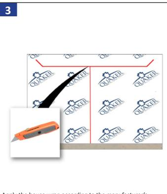
Apply the house wrap according to the manufacturer's instructions and cut T-pattern opening as shown above. Cut top flap angles at 45 degrees and 1" longer than the width of flashing tape being used.
