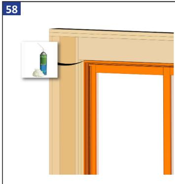
Insulate the gap between the door and framing with minimally expanding spray foam, and seal the entire interior perimeter with sealant.
