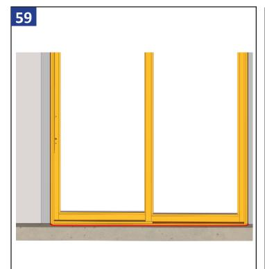
Apply a continuous bead of sealant at the exterior base of the sill. Be sure to not block the weeps on the bottom of the sill.
