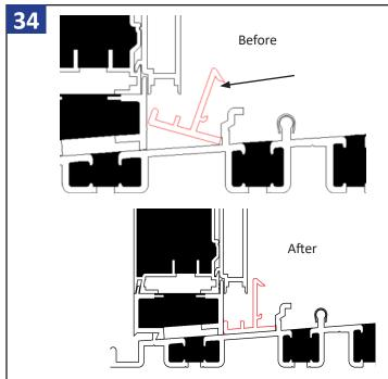
Lock the panel sill in place with three sill compression locks (Part #: M24381-PCS). Set fixed panel sill compression lock down in the track and then take a flat head screw driver and pop into place as shown above.
