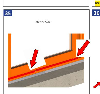
Take baffle(Part #: QWP-50x75X60), cut to length, then press the baffle down between compression locks and the frame. The baffle will run full length.
