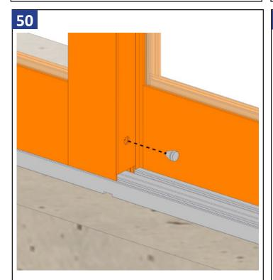
Once all panels have been adjusted install the panel bumpers into each roller adjustment hole.
