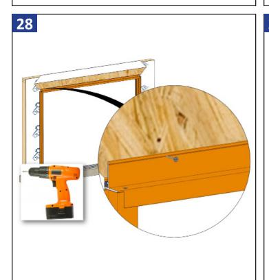
**NAIL FIN ONLY!**Fully tighten the fasteners down now to hold the frame in place. All fastener locations are to shimmed between framing and condition
