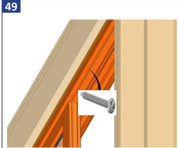
Slide the panel over to finish drilling and installing fasteners in the head closure.
