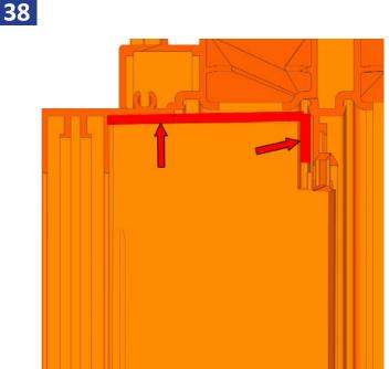
Press fixed panel weep baffle (Part #: QWP-50x75X60) in above the top of the fixed panel between the panel and frame. Then silicone and tool in smoothly with a putty knife.
