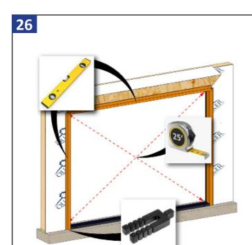
Square, level, and plumb the frame. Adjust shims as needed until diagonal measurements are within 1/8". Shim behind the header and jambs as necessary.
