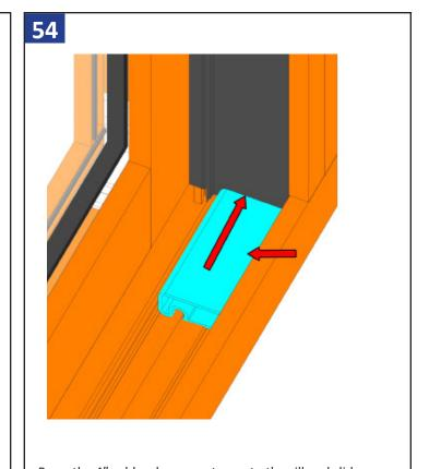
Press the 4" rubber bumper stop onto the sill and slide over to the frame.
