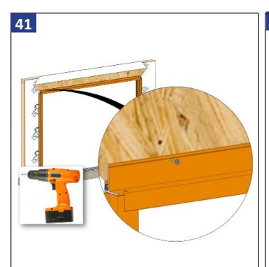
**NAIL FIN ONLY!** Fully fasten the screws down now to hold the frame in place.
