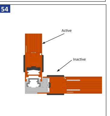
Once all the panels are installed close the panels. Make sure the inactive and active panels lock as shown above.
