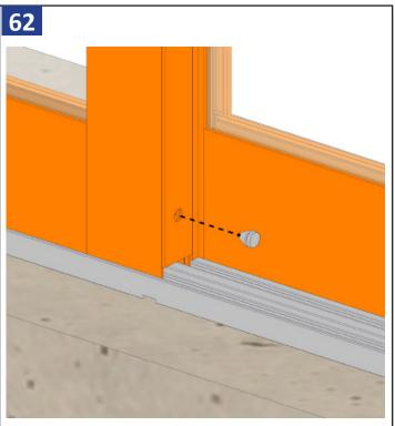
Once all panels have been adjusted install the panel bumpers (Part #: 9309K86) into each roller adjustment hole.
