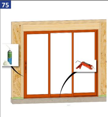
Insulate the gap between the door and framing with minimally expanding spray foam, and seal the entire interior perimeter with sealant. On the interior side of the middle panels, take the panel pickups (Part #: M25296-PCS) and #10 screw (Part #:MF10AX1)that is provided. Take screws and attach the pickups. Install the panel pickup where the holes are already fabricated on the interior side of the door. wd
