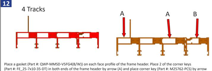
(Part #: FE\_25-7x10-35-DT) in both ends of the frame header by arrow (A) and place corner key (Part #: M25762-PCS) by arrow (B). Then join to both frame jambs to head. Trim weather strip flush to both ends. Step 11, figure B shows the 90 degree angled joint, place 1 gasket (Part #: QWP-MMSD-5FG10(B/W)) on the face. Then slide 2 corner keys (Part #: M25763-PCS) A and one (Part #: M25764-PCS) in B as shown above into the angled head. (NOTE: These keys are for installation purposes only.)
