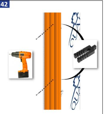
Fully fasten the screws down now to hold the frame in place. The holes through the center track of the header & jambs, typically 6" from ends and 2' on center for fasteners. Shim tight to sill pan.
