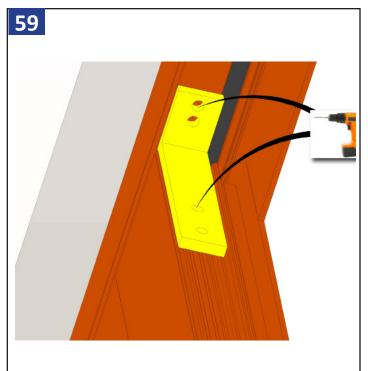
Take the **Fixed Panel Bracket**, slide it to the head drill holes for the tri-wing screws.
