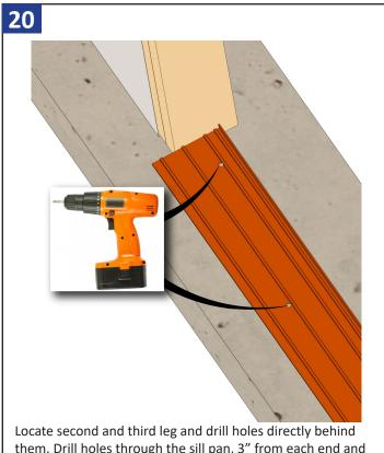
them. Drill holes through the sill pan, 3" from each end and then 14" on center for the length of the pan, alternating between the 2 tracks. Blow out the debris on the sill pan. (Drill bit size is based off screw size) 21
