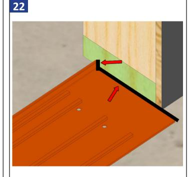
Silicone along the wall and upturned leg. Be sure to tool in the sealant.
