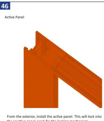
From the exterior, install the active panel. This will lock into the inactive panel. Look for the locking mechanism. \*Note orientation of interlock rails when choosing panels. \*Note glazing beads are to the interior side.
