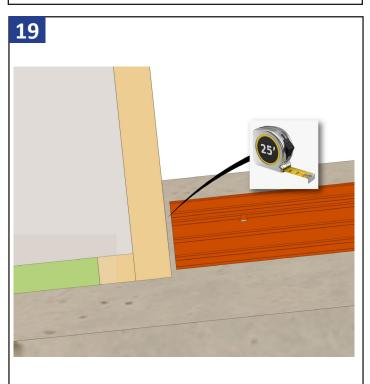
Allow a 1/4" gap between the rough opening and the sill pan.
