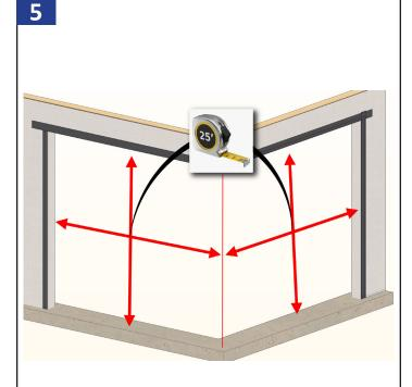
Measure and verify the rough opening is sized correctly. The rough opening should be 3/4" wider and 1/2" taller than the unit. Allow additional space for flashing thickness, installation clips, joining components, and their fasteners.
