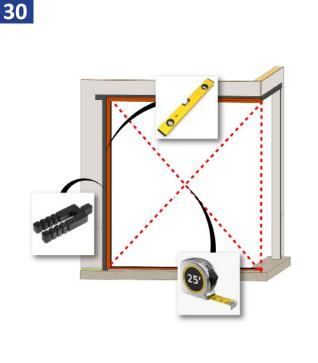
Square, level, and plumb the frame. Adjust shims as needed until diagonal measurements are within 1/8". Shim behind the header and jambs as necessary.
