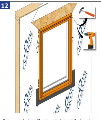
Temporarily fasten with a single fastener at the top of one jamb side as shown.
