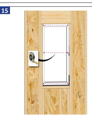
Check that the window is not bowed. Adjust shims as needed unit measurements are within 1/8".
