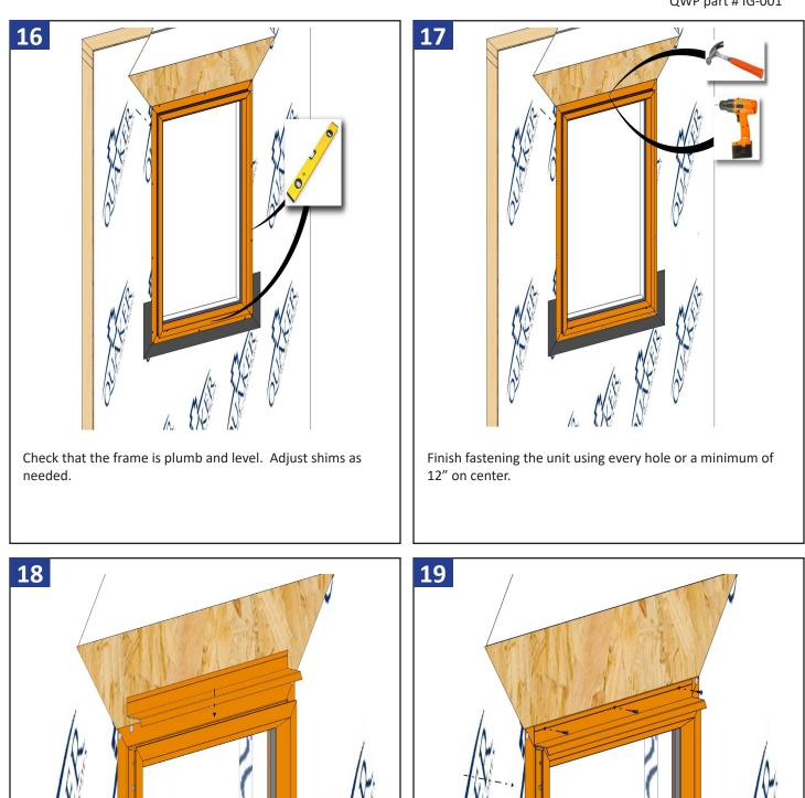
Apply the head flashing to the top edge of window as shown below.
