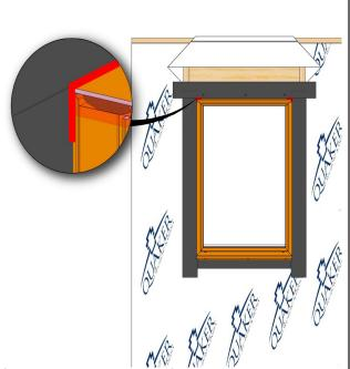
Apply flashing tape over the head flashing, overlapping the side flashing as shown, covering any seam or gap in the nailing fin at the corners. Smooth using a J-roller. Put sealant at top corners of flashing tape.
