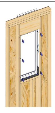
Shim at the sides of the window, and at the check rail locations. Never shim at the head.
