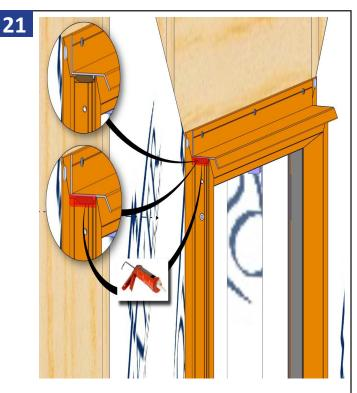
Use backer rod and sealant to seal both ends of the head flashing and window as shown above.
