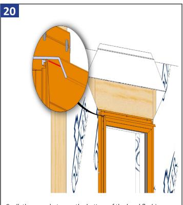
Caulk the seam between the bottom of the head flashing and top of the window.
