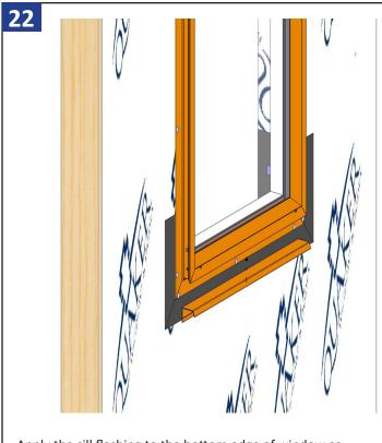
Apply the sill flashing to the bottom edge of window as shown above.
