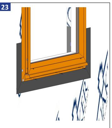
Fasten the sill flashing tight against the bottom of the window with self tapping screws as shown above.
