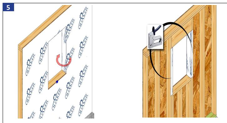
Fold the house wrap to the interior and staple it to the interior framing. Tape the house wrap at the bottom of the opening as shown.
