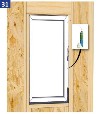
Fill interior 1/3 of the cavity using low expanding foam or loose insulation.
