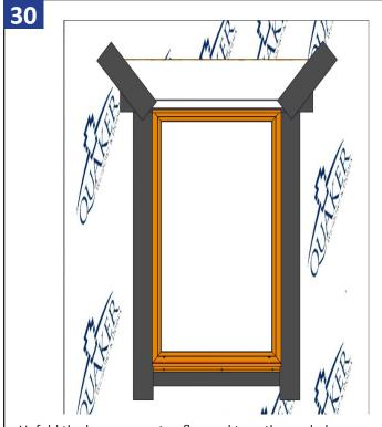
Unfold the house wrap top flap and tape the angled seams as shown above.
