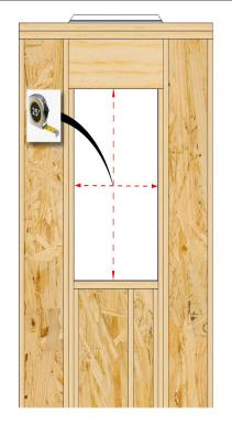
Measure and verify the opening is sized correctly. The rough opening should be a minimum 1/2'' (but not to exceed 1'') wider and taller than the unit. Allow additional space for flashing thickness, installation clips, joining components, and their fasteners.
