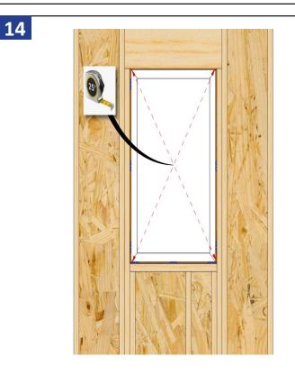
Check that the window is square. Adjust shims as needed to assure unit diagonal measurements are within 1/8".
