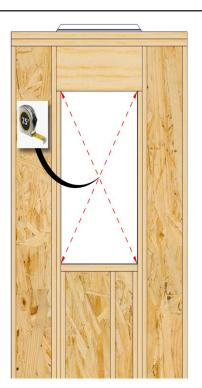
Check that the opening is square. The diagonal measurements need to be within 1/8" of each other.
