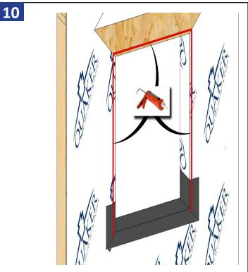
Apply a continuous 3/8" sealant bead at the sides and the top of the opening, no more than 1/2" from the edge of the opening as shown. **Sealant needs to line up with nail hole slots.** No sealant needed at the bottom or use a **non continuous** bead to allow for drainage.
