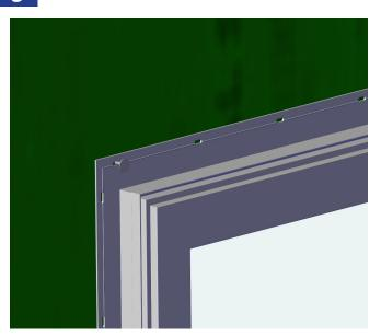
Make sure window is closed and locked before setting the window. Center and set the window into the rough opening, making sure there are equal gaps on both sides of the window.
