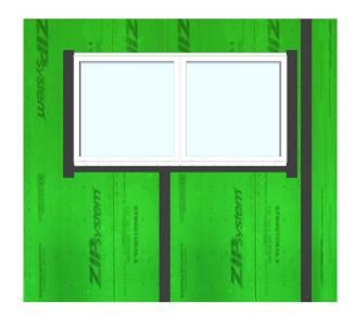
Cut two pieces of flashing tape for jamb flashing extending 1" above window head flange and 4" to 6" below bottom edge of sill flashing. Use roller to press tightly along sides of window frame.
