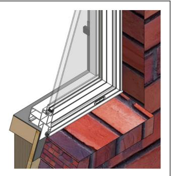
After siding or wall exterior is complete, apply backer rod and sealant between the window frame and exterior finish material on all four sides of unit. Make sure to clean all surfaces before applying sealant.
