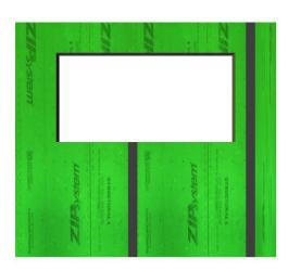
Inspect the joints of the water resistant sheating. Joints must be sealed according to the sheating manufacturer's instructions. Quaker assumes no responsibility for the design, quality or durability of the sheating system or its joints.
