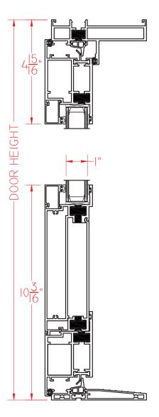
All drawings shown without nailing fin and square glazing stops
